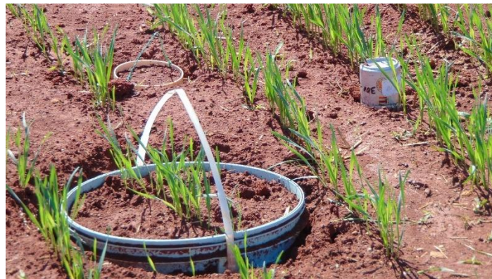
Supplementary Fig 2. Lysimeter, small-lysimeter and access tube installed in the experimental plot.
