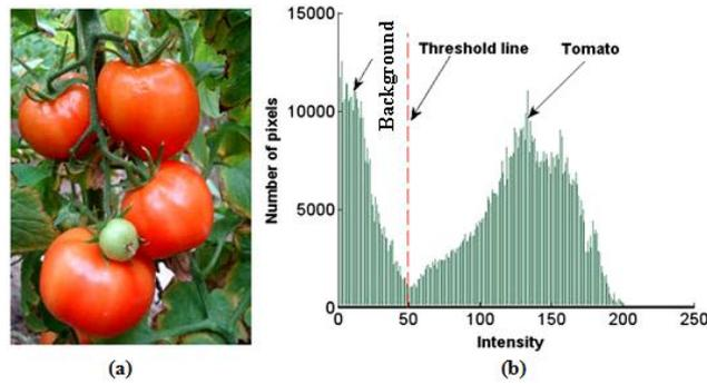
**Fig 1.** The corresponding Histogram to Drg relation: **a** original image. **b** corresponding histogram, it can be observed that threshold line has successfully separated tomatoes (placed in the right of the valley) from the background (placed in the left of the valley) and so this issue ensure removing the background.
