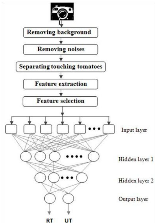
**Fig 4.** Flowchart of process of ripe tomato recognition: first, color images of tomato were acquired. Background of the image was removed by threshold segmentation. All noises were removed and glued tomatoes were separated based on morphology operation. Wavlet features were extracted for each tomato and then the most effective features were selected. The selected features were defined as ANN input and finally ripe and unripe tomato were recognized using trained ANN
