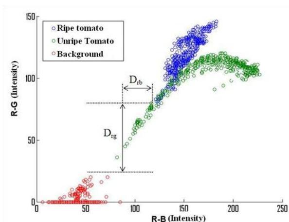
**Fig 5.** Pixel distribution diagram of the ripe tomato, unripe tomato, and background (Arefi et al., 2011);  $D_{rb}$  show difference between red and blue components, and subtraction of red from green component is shown by  $D_{rg}$ .
