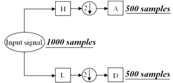
**Fig 7.** Decomposition of signal by two filters: Input signal is broken down into two frequencies by two low-pass and high-pass filters. In continuous, down-sampling reduces samples of each out-put signals to half (Misiti et al., 2002).
