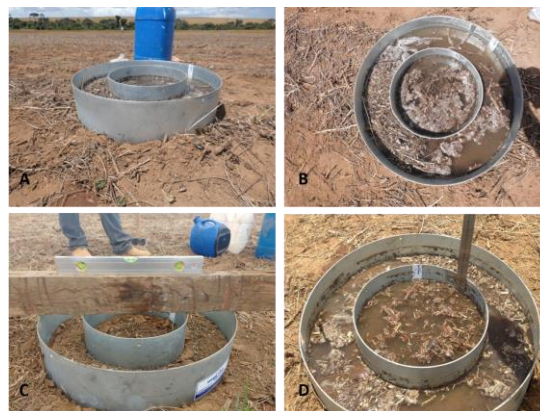
Figure 10. Installation of concentric infiltration rings for monitoring soil infiltration in areas of (A and B) pasture and (C and D) agriculture.
