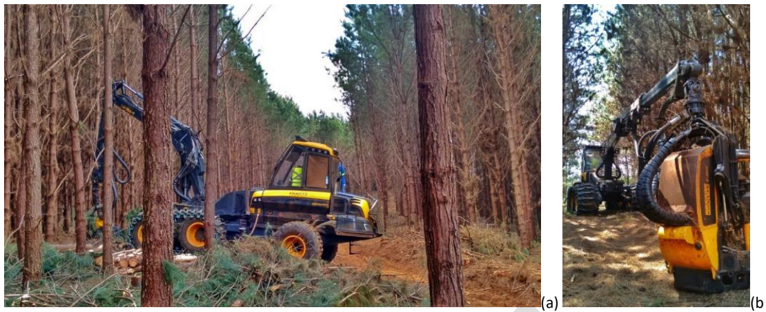
Fig 4. Ponsse beaver harvester at work (a). Processor head (b).
