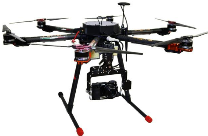
Fig 2. UAV exacopter, model: Novex, brand "IDS" with Sony Ilce 6000 camera.
