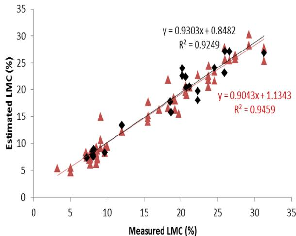
**Fig 6.** Correlation between estimated LMC with NN method and real LMC in training ( $\blacktriangle$ ) and testing ( $\blacklozenge$ ) step.
