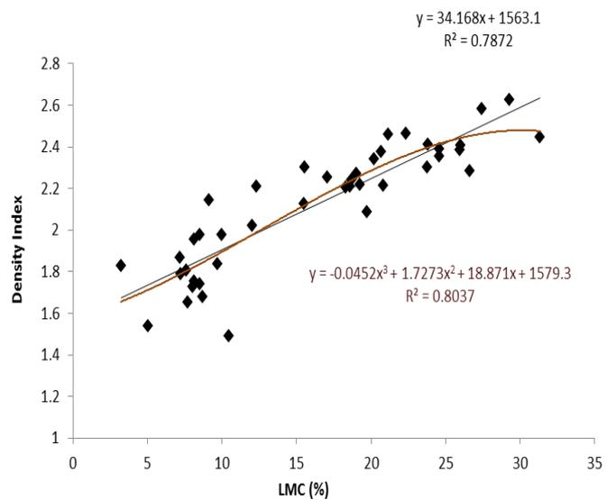
**Fig 5.** The LMC and density index correlation obtained by image processing
