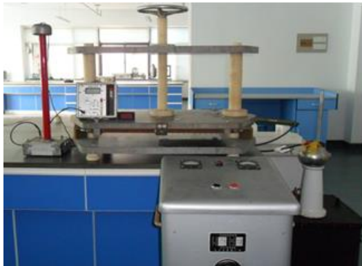
Fig 2. Photo of high voltage electric field treatment equipment.
