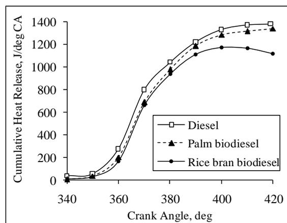
**Fig 4.** Variation of cumulative heat release with crank angle at full load conditions shows the cumulative heat release for same crank angle duration for diesel, palm biodiesel, and rice bran biodiesel.
