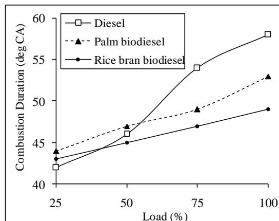
**Fig 7.** Variation of combustion duration with load for diesel, palm biodiesel, and rice bran biodiesel.
