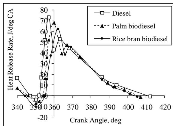
**Fig 3.** Variation of heat release rate with crank angle at full load conditions shows the magnitude and occurrence of peak heat release rate for diesel, palm biodiesel, and rice bran biodiesel.
