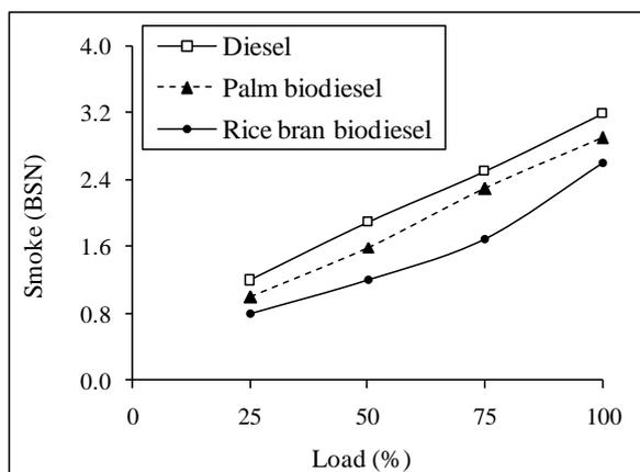
**Fig 9.** Variation of smoke with load shows the magnitude of smoke density at various engine loads for diesel, palm biodiesel, and rice bran biodiesel
