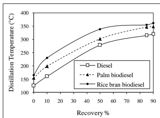
**Fig 1.** Distillation temperatures of diesel, palm biodiesel, and rice bran biodiesel to compare their volatility characteristics
