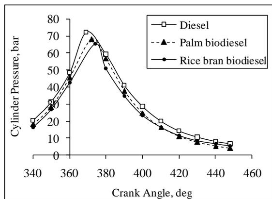
**Fig 5.** Variation of cylinder pressure with crank angle at full load conditions shows the magnitude and occurrence of peak pressure for diesel, palm biodiesel, and rice bran biodiesel.
