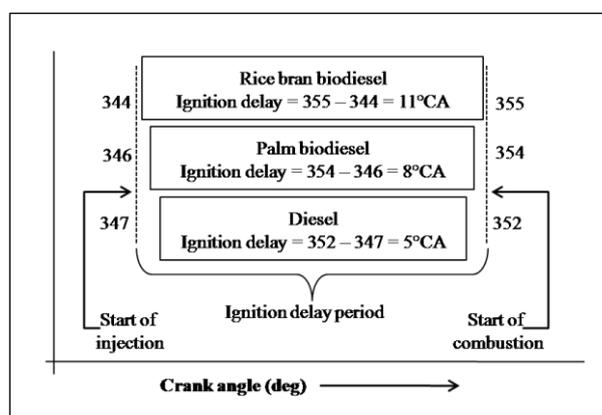
**Fig 2.** The actual SOI, ignition delay, and start of combustion of test fuels at full load conditions.
