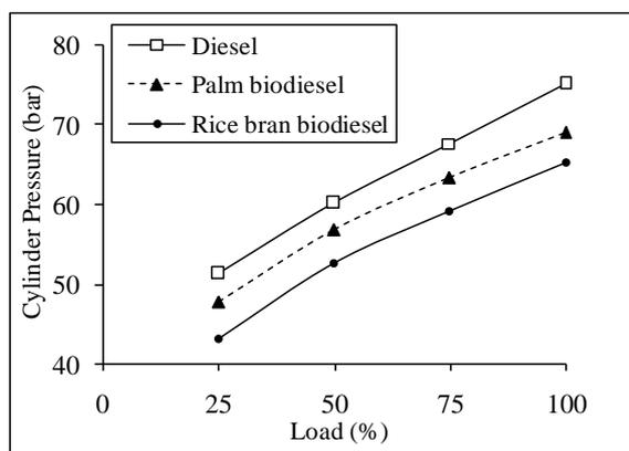
**Fig 6.** Variation of peak pressure with load shows the magnitude of peak pressure at various engine loads for diesel, palm biodiesel, and rice bran biodiesel.
