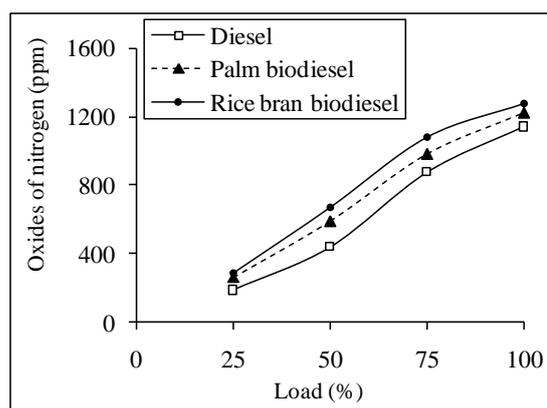
**Fig 8.** Variation of oxides of nitrogen with load shows the magnitude of NO<sub>x</sub> emissions at various engine loads for diesel, palm biodiesel, and rice bran biodiesel.
