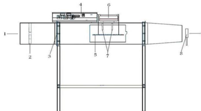
**Fig 1.** Schematic diagram of the convective drying equipment (1) Air inlet; (2) Fan; (3) Heaters; (4) Temperature and air flow velocity controlling; (5) Perforated tray; (6) Digital balance; (7) Relative humidity sensor and thermocouple to data logger; (8) Digital anemometer; (9) Air outlet.
