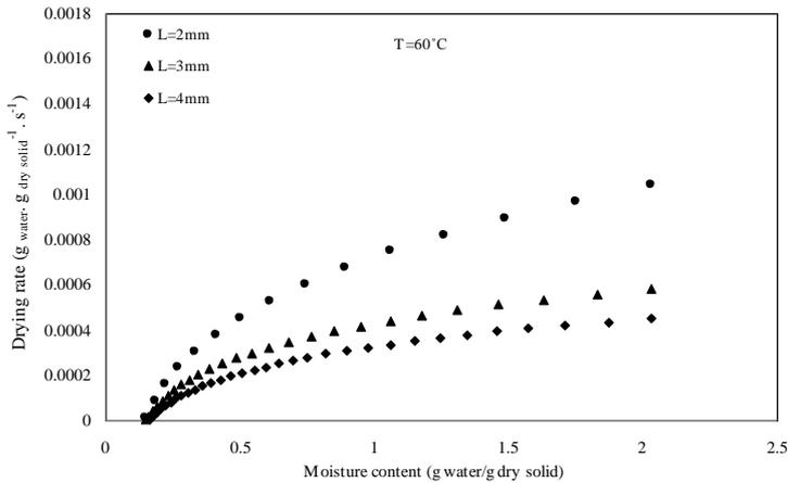
**Fig 4.** Drying rate vs. moisture content of garlic slices at air temperature of 60°C and slice thicknesses of 2, 3 and 4 mm
