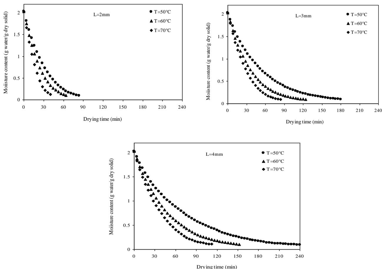
**Fig 2.** Drying curves of garlic at different air temperatures and sample thicknesses
