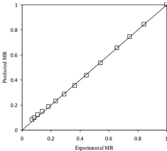
**Fig 5.** Predicted moisture ratio by Weibull model vs. experimental values at the air temperature of 55°C and slice thickness of 2.5 mm
