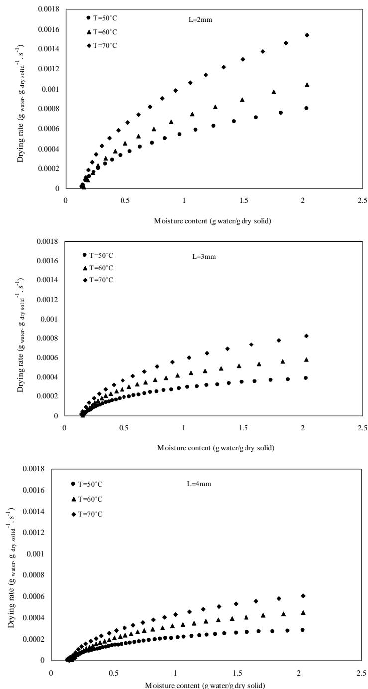
**Fig 3.** Drying rate vs. moisture content of garlic slices at different air temperatures and slice thicknesses.
