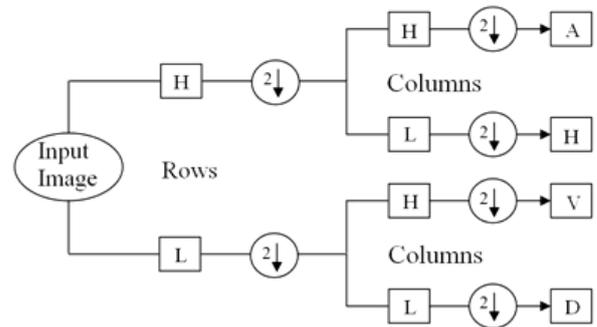
**Fig 8.** Decomposition of image with a filter bank: Input image breaks down into one approximation (A) and three details including horizontal (H), vertical (V) and diagonal (D) (Gonzalez and woods, 2004).
