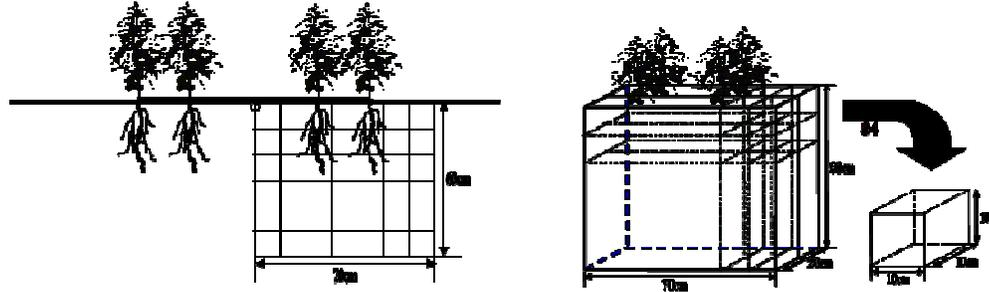
**Fig 2.** Schematic illustration of the root excavation method. A monolith method was used to harvest roots at 40, 65, 82, 96, 110, 125, and 160 DAS. Soil cubes with 10 cm sides ( $1000 \text{ cm}^3$ ) were dug individually in a soil volume of 70 cm  $\times$  20 cm and to a depth of 60 cm surrounding four plants. The total number of monoliths excavated for the four plants was 84.
