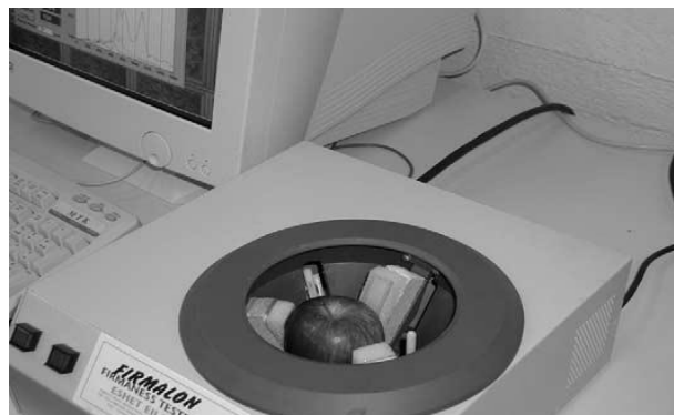
Fig 8. The FIRMALON used three piezoelectric sensors to measure fruit firmness (shmulevich, 2003).
