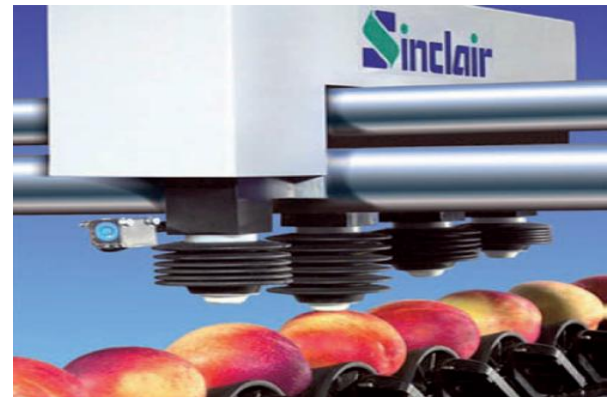
Fig 2. The Sinclair sensor hits the fruit by air pressure and captures the impact signal (Howarth, 2002).
