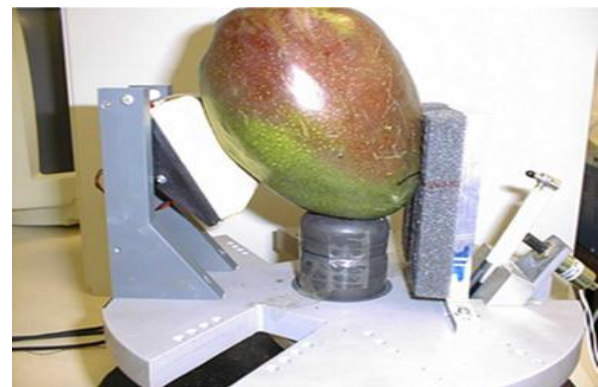
Fig 4. A low-mass impact apparatus used a 4-mm diameter hemispherical aluminum tip to produce the impact signal (Shmulevich, 2003).
