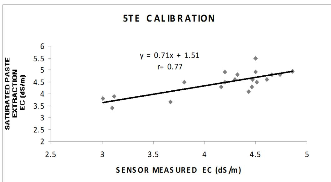
**Fig 1.** Sensor measured electrical conductivity (EC) was linearly regressed against conventional saturated paste extract electrical conductivity (EC).
