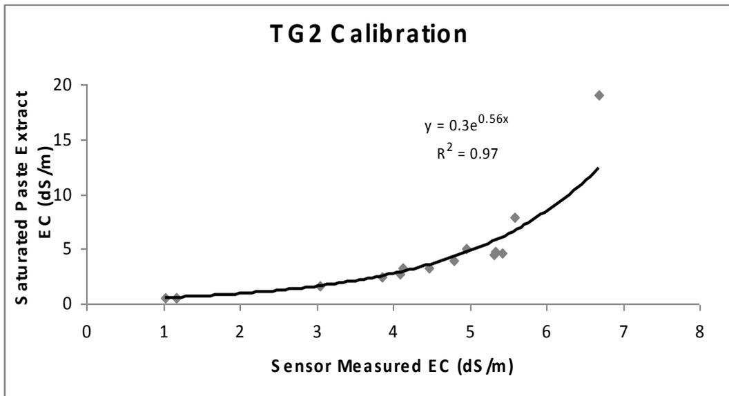
**Fig 6.** Non-linear regression of sensor measured electrical conductivity (EC) and conventional saturated paste extract electrical conductivity (EC).
