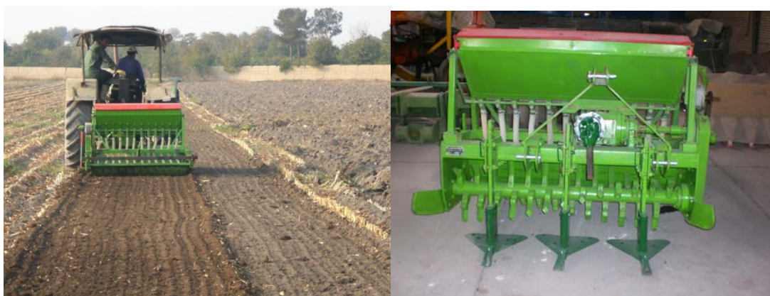
Fig 1. Multi-task machine during reduced tillage operation
