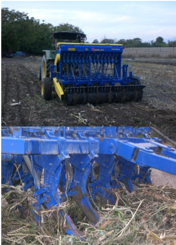
Fig 2. Direct sowing machine during No-Till operation
