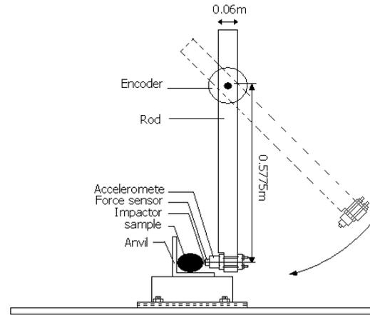
**Fig 7.** Schematic representation of the pendulum rod and anvil. The positions of the different sensors and of the impacted body “fruit” are indicated.
