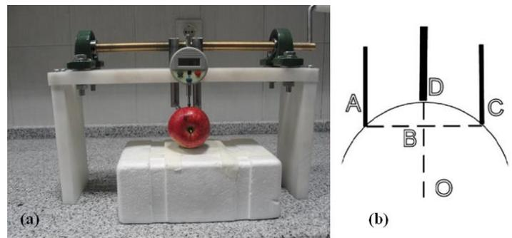
**Fig 9.** (a) General view of the curvature meter and (b) schematic representation of geometry to calculate the radius of curvature of the apple fruit.
