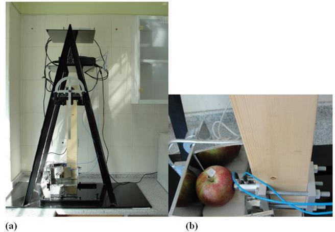
**Fig 8.** (a) General view of the pendulum device for measuring impact force and impact velocity of the apple fruit and (b) the anvil and rod of the pendulum at beneath the frame.
