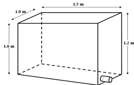
**Fig 1.** Schematic of the lysimeter used to collect field data
